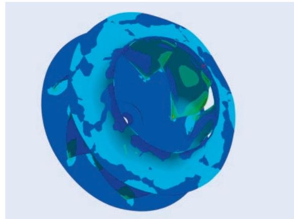
Impeller strength calculation using the finite element method FEM.
